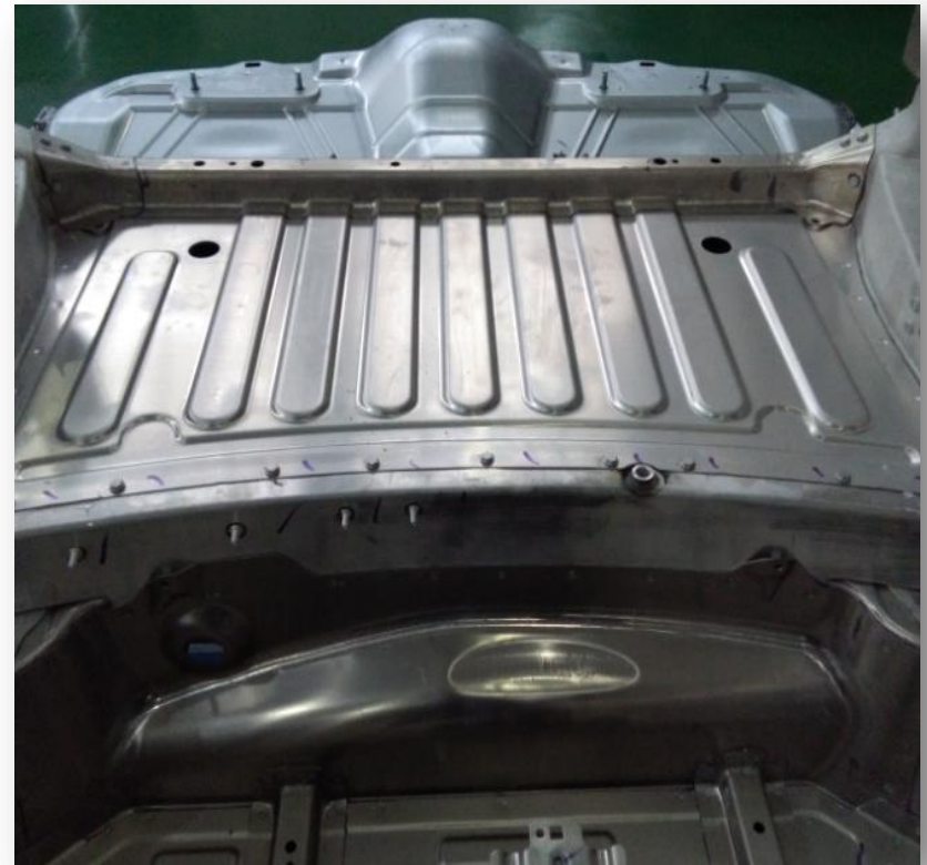
back cockpit floor and trunk 后驾驶舱地板和后备箱
