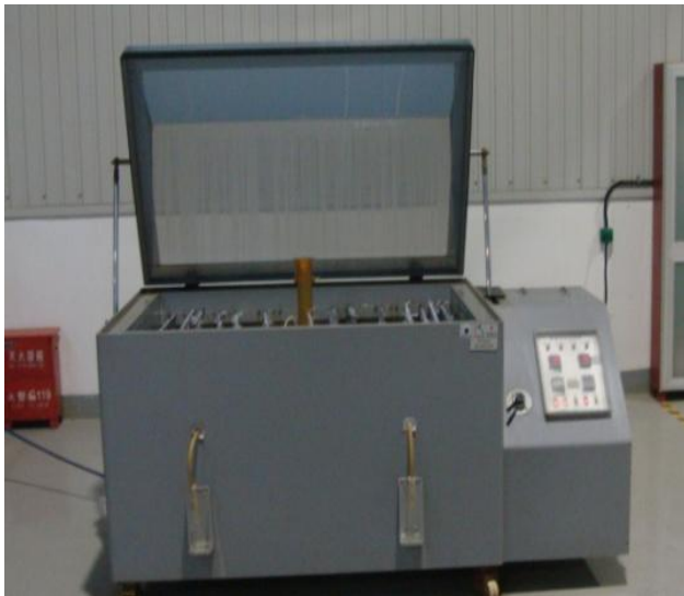
Salt spray tester 盐雾实验设备
