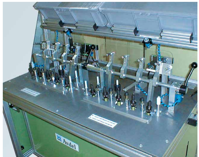
10 placing heads to assemble automotive sealing strips
