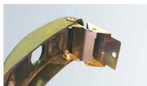
Composite material latch for wheel cover
