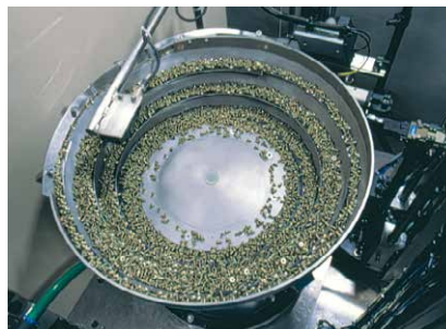
Fasteners fed via a vibrating bowl
