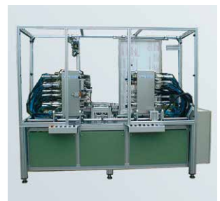
23 placing heads to assemble a computer chassis
