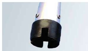
Composite material latch for wheel cover
