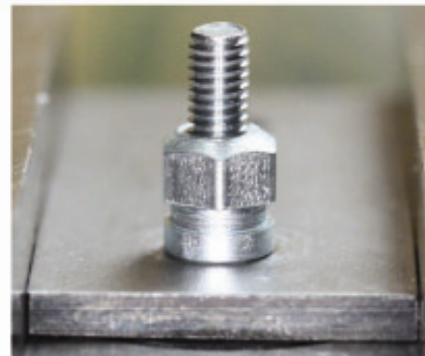
Figure 1 M4 nut about to be tested.
